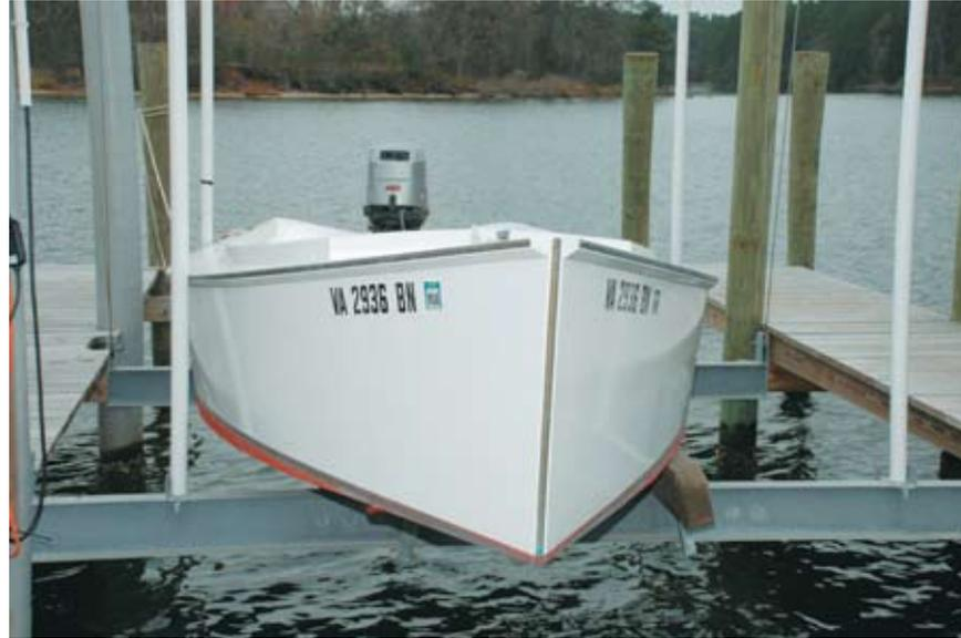
**Though it has the smooth look of a new fiberglass boat, this is one of the Cockrell’s PVC skiffs. The boat was built with 1-inch and 1 1/4-inch PVC panels that are held together with glue.**
